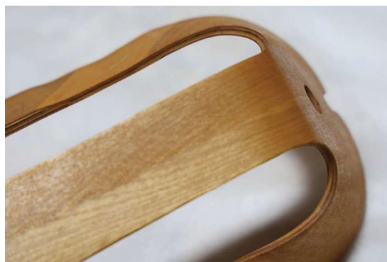
Fig. 8 Laminated edge at curved section / 湾曲部の積層端面
