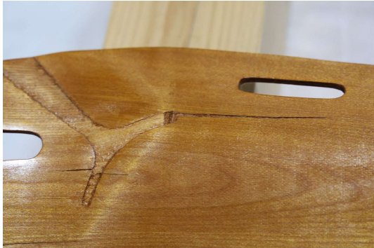
OM-PD-LS-001-P086 局所亀裂・接合部近傍（拡大 8） Localized crack near a joint (close-up 8) Source: 0R9A0094.JPG
