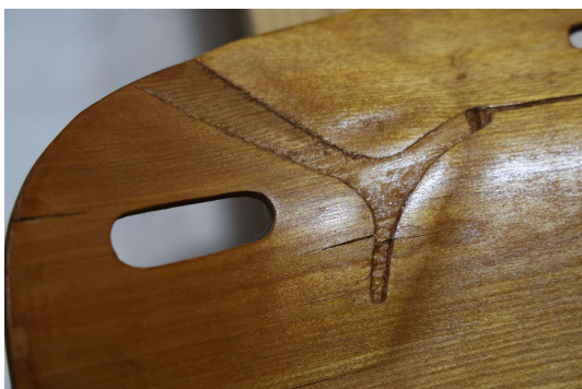
OM-PD-LS-001-P080 局所亀裂・接合部近傍 (拡大 2) Localized crack near a joint (close-up 2) Source: 0R9A0088(1).JPG
