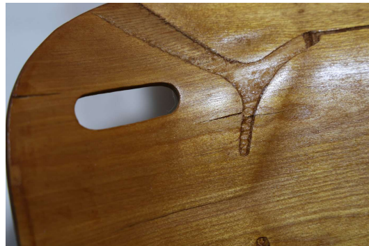
OM-PD-LS-001-P079 局所亀裂・接合部近傍 (拡大 1) Localized crack near a joint (close-up 1) Source: 0R9A0087.JPG
