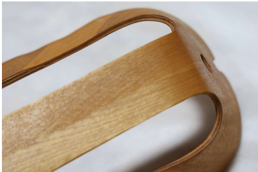
OM-PD-LS-001-P090 積層断面・外周縁・開口部（接写 3） Lamination section, perimeter edge and opening (close-up 3) Source: 0R9A0106(1).JPG
