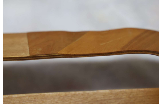
OM-PD-LS-001-P089 積層断面・外周縁・開口部（接写 2） Lamination section, perimeter edge and opening (close-up 2) Source: 0R9A0105.JPG
