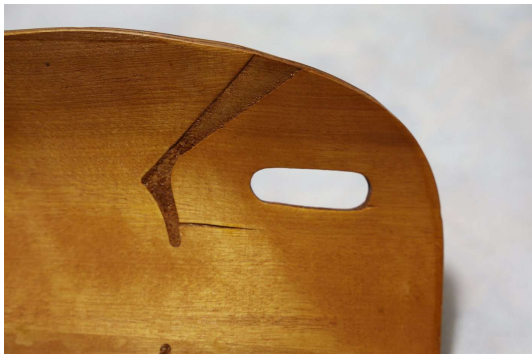
OM-PD-LS-001-P092 局所亀裂・接合部近傍（補足拡大 1） Localized crack near a joint (supplementary close-up 1) Source: 0R9A0110(1).JPG
