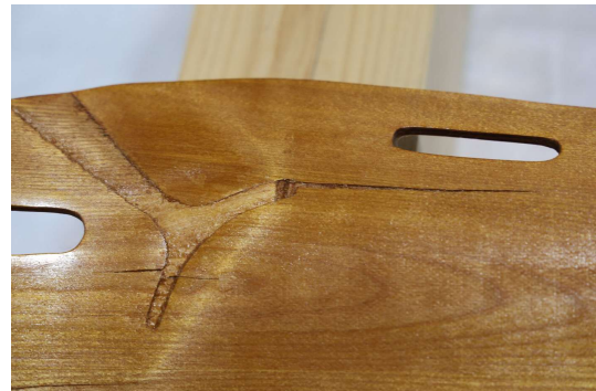
OM-PD-LS-001-P085 局所亀裂・接合部近傍（拡大 7） Localized crack near a joint (close-up 7) Source: 0R9A0093(2).JPG
