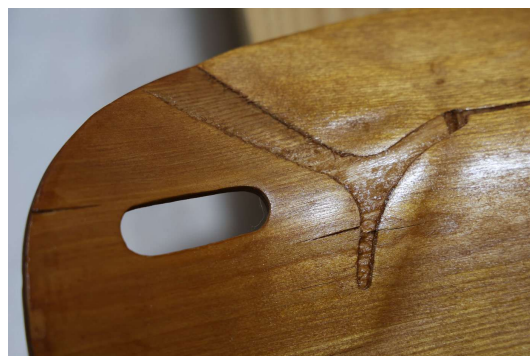
OM-PD-LS-001-P081 局所亀裂・接合部近傍 (拡大 3) Localized crack near a joint (close-up 3) Source: 0R9A0089.JPG
