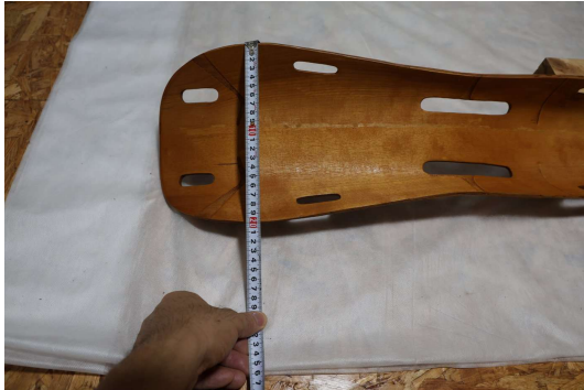
OM-PD-LS-001-P101 上部幅計測・約 199 mm (方向違い 1) Upper-section width measurement, approx. 199 mm (angle 1) Source: 0R9A0147.JPG
