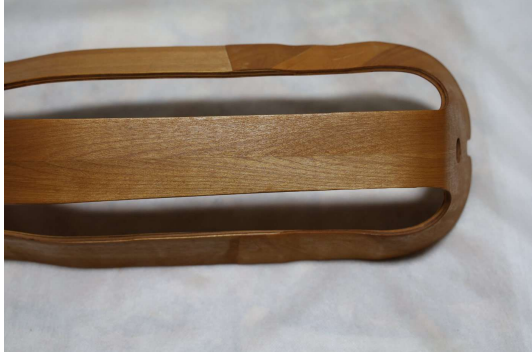
OM-PD-LS-001-P088 積層断面・外周縁・開口部（接写 1） Lamination section, perimeter edge and opening (close-up 1) Source: 0R9A0101.JPG
