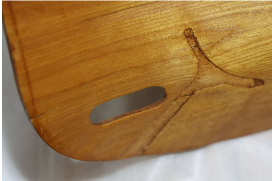
OM-PD-LS-001-P082 局所亀裂・接合部近傍（拡大 4） Localized crack near a joint (close-up 4) Source: 0R9A0090(1).JPG
