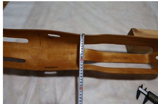
OM-PD-LS-001-P100 中央部幅計測・約 137 mm Central-section width measurement, approx. 137 mm Source: 0R9A0145.JPG
