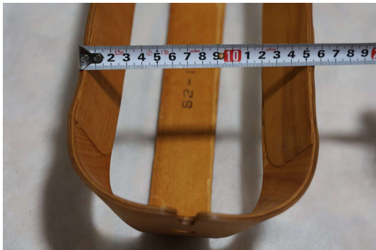
OM-PD-LS-001-P099 下部幅計測・約 155 mm (方向違い 2) Lower-section width measurement, approx. 155 mm (angle 2) Source: 0R9A0140.JPG
