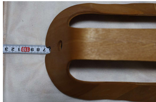
OM-PD-LS-001-P104 全長計測・1,068 mm (読取方向違い 2) Overall-length measurement, 1,068 mm (reading angle 2) Source: 0R9A0154.JPG
